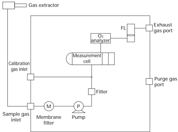
Two optical lines (3 to 4-component gas sampling system diagram): Type ZSVS
