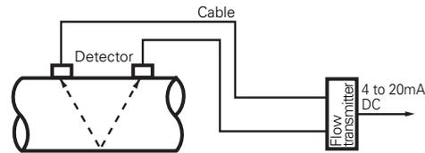
(2) When Z method is used for mounting
