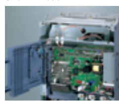
The inverter's mounting screws and power connector can be removed from the front.
